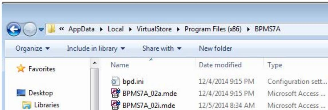
When you run the installation program, as long as no one is running the BPMS application, the installation program will delete the files with extension .MDE. The next time the user runs the application, the latest update will be copied to their local profile folder.
